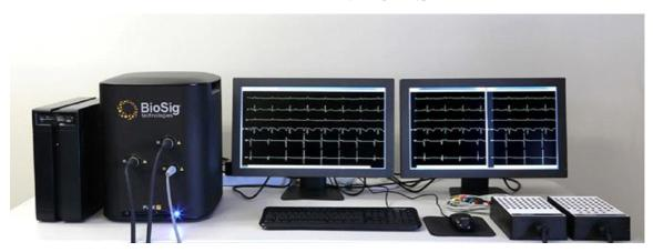
The current PURE EP System prototype
